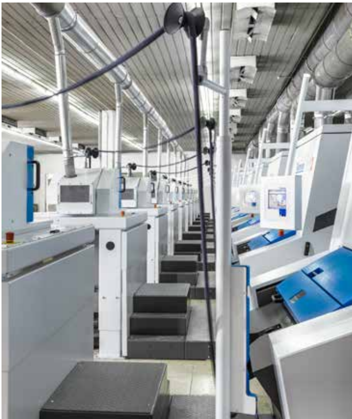
Here reclaimed fibers (recycled jeans) are carded for rotor spinning. The passage between cards and IDF 2 makes operation much easier for the staff.
