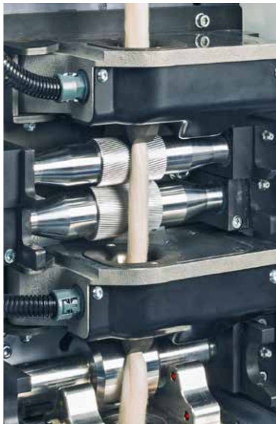
Sensor to determine sliver count (top) and quality sensor (bottom)
