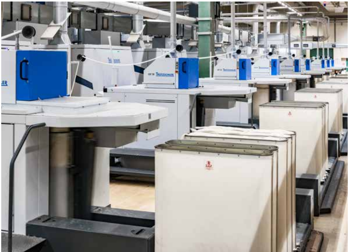
A rectangular can has almost twice the capacity of a traditional can with 450 mm diameter. Another advantage of rectangular cans is the easier implementation of an automatic can transport.
