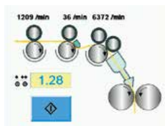
AUTO DRAFT: Automatic optimization of break draft and simple break draft setting Page 20
