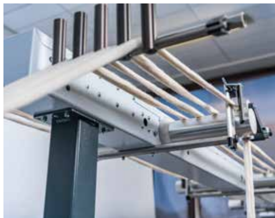
Individual sliver monitoring in the feed area of the draw frame
