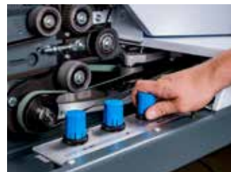
Pneumatic top roll load: Precise pressure settings via the display Page 10
