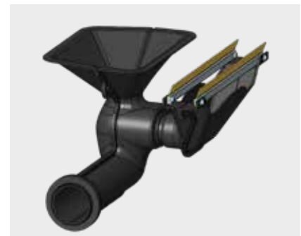
The suction elements are individually simulated to optimise flow and are made of robust plastic.
