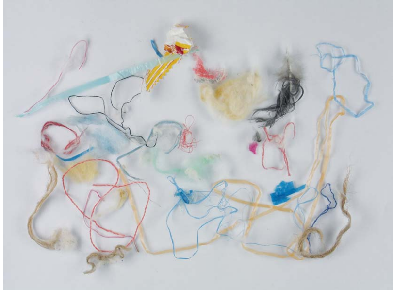
Examples of detected foreign parts after conversion to Retrofit KIT SC1. The small thread-shaped parts and even parts in pastel shades can be clearly detected.
