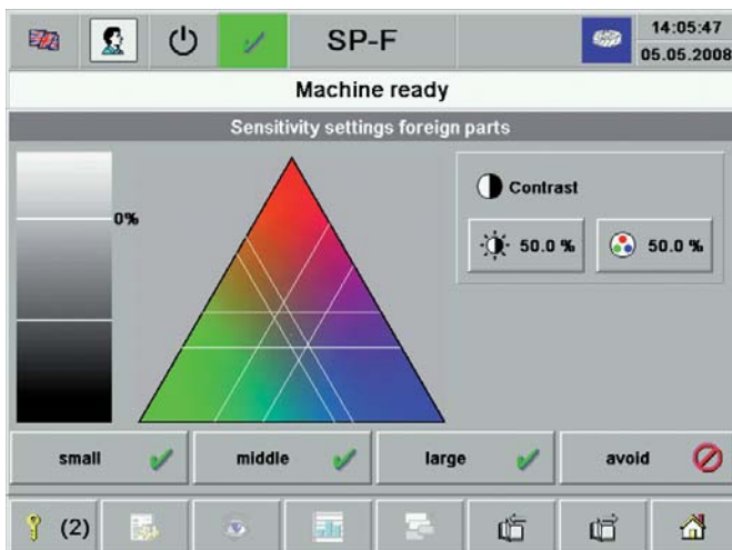
Setting sensitivity with brightness and colour contrast
